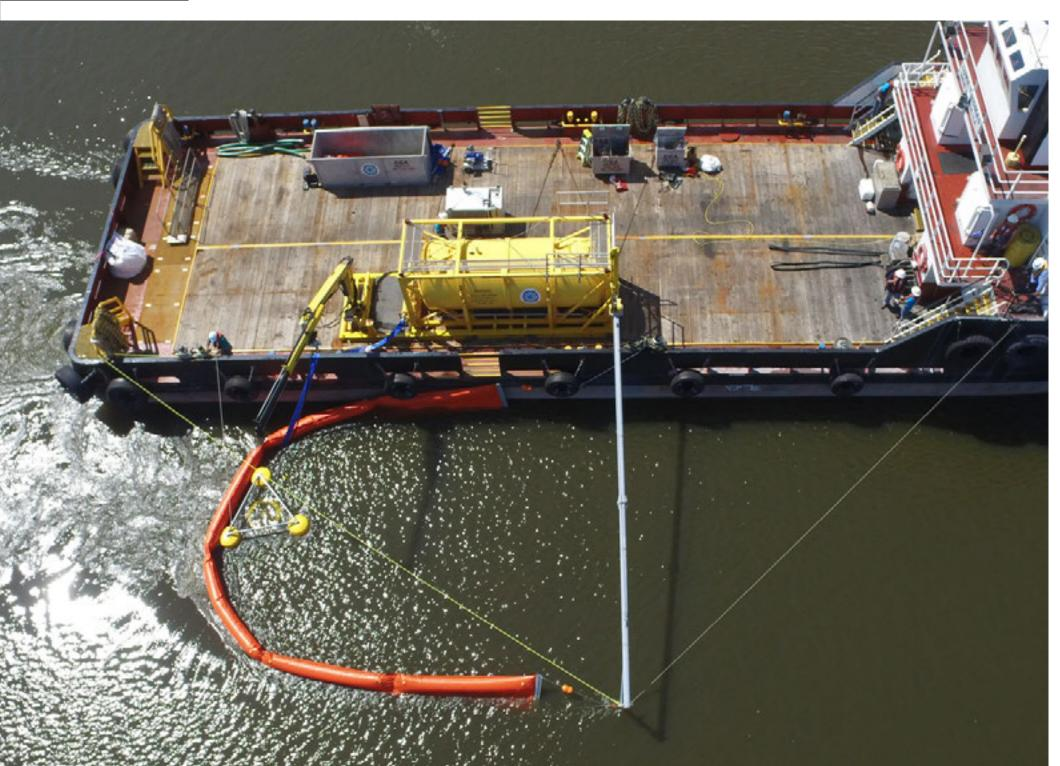
These steps are for the loadout, deployment and recovery of the FRU skimming equipment deployed on the back deck of a utility vessel and using the outrigger booming configuration.
