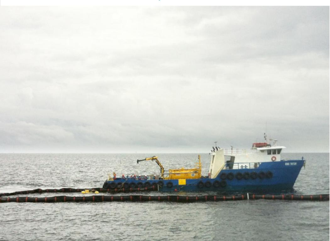
These steps are for deployment and recovery of offshore inflatable boom in conjunction with the FRU skimming equipment to increase the encounter rate with oil by using an enhanced "J" booming configuration.
